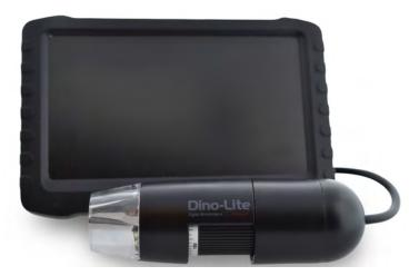
For mobile applications the AMK4112TL-D15 is a great combination of a Dino-Lite digital microscope with long working distance, and a portable digital recorder (D15). The long working distance of up to 15 cms makes it possible to work under the microscopes (precision assembly/soldering etc.) The recorder has a 5 inch LCD panel, and pictures and video can be recorded on an included 4GB SD-Card.
