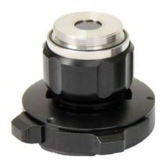
C-mount adapter for rigid endoscopes with a focal length of 25mm. This C-mount adapter connects to rigid, straight through endoscopes with max. 32mm ocular diameter.
