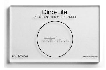
The CS-30 is a glass calibration slide that can be used to calibrate your Dino-Lite digital microscope or to be used with the Dino-Eye eyepiece cameras. The total length is 10mm (10.000um) and the smallest gradation on the slide is 0.1mm (100um).
