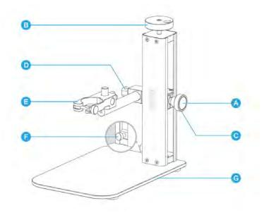
A: Quick Release Button B: Fine-Focus Knob C: Anti-Backlash Lock D: Arm Screw E: HD-M2A Holder
