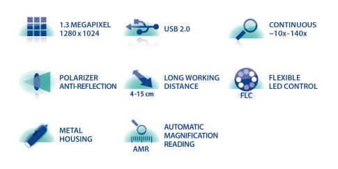
The AMR function automatically detects and displays the magnification of the Dino-Lite. The magnification is displayed within the Dino-Lite software and stored with the captured picture and simplifies the measuring process. Because of the built-in polarization filter this model is ideal when working with shiny or reflective objects such as metal, plastic, glass, jewelry, electronics, etc.
