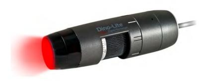
The Dino-Lite AM4115T-DFRW digital microscope is optimized for research and viewing fluorescent objects by using 620nm excitation LEDs. It has a long-pass type 650nm emission filter that is designed to observe a wide range of fluorophores with applications in developmental biology, pathology, and anatomy.
