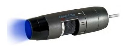
The Dino-Lite AM4115T-GFBW digital microscope is optimized for research and viewing fluorescent objects by using 480nm LEDs. It has a 510nm emission filter that is designed to observe including but not limited to GFP (green fluorescent protein).
