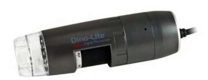
The AM4115-FIT has special lighting with LED's emitting IR light around the 850 nm spectrum.
