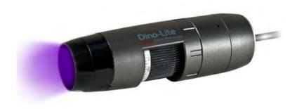
The Dino-Lite AM4115T-CFVW digital microscope is optimized for research and viewing fluorescent objects by using 400nm near UV excitation LEDs. It has a long-pass type 430nm emission filter that is designed to observe a wide range of fluorophores with applications in developmental biology, pathology, and anatomy.
