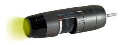
The Dino-Lite AM4115T-RFYW digital microscope is optimized for research and viewing fluorescent objects by using 575nm excitation LEDs. It has a long-pass type 610nm emission filter that is designed to observe a wide range of fluorophores with applications in developmental biology, pathology, and anatomy.
