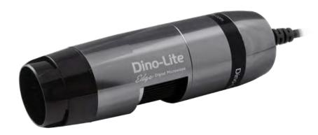
The Dino-Lite AM7115MT-FUW is part of the Dino-Lite special light range. This model has two types of LED lights that are switchable between white and UV light. The UV LEDs are near UV-fluorescent LEDs with a spectrum of 375nm. This model offers a standard working distance, a wide magnification range from 20 – 220x and comes with a high quality 5 megapixel Edge sensor.
