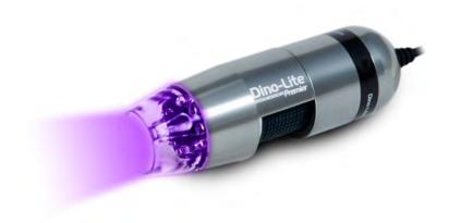
The VW series has two types of LED lights that are switchable between white and UV light. This model has a long working distance and a filter to filter out the returning UV light so that an image with natural colors can be obtained. The aluminium housing offers enhanced protection and durability and has the best look and feel.
