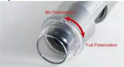
Rotate the ring to adjust the amount of polarization you require.
