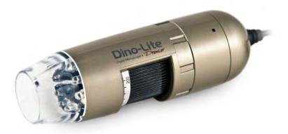
The VW series has two types of LED lights that are switchable between white and UV light. This model has a filter to filter out the returning UV light so that an image with natural colors can be obtained.
