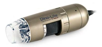
The VW series has two types of LED lights that are switchable between white and UV light. This model has a long working distance and a filter to filter out the returning UV light so that an image with natural colors can be obtained.
